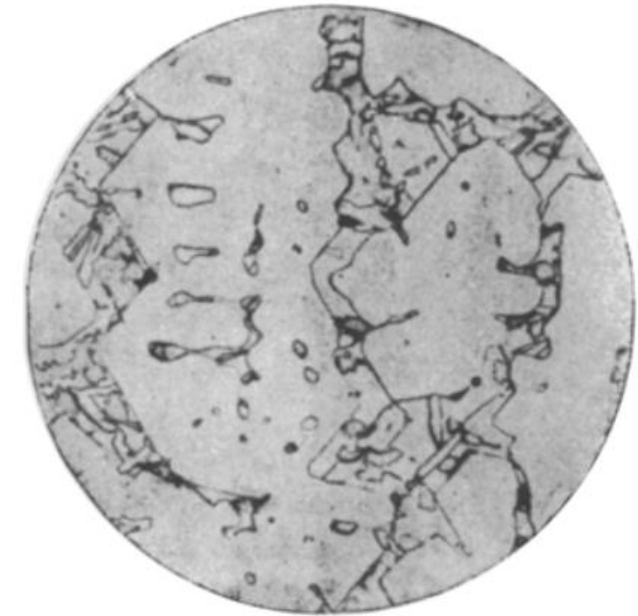
Fig. 2. Microstructure of the alloy Nb_3Ni_2Si (composition of materials used). Magnification 200.
